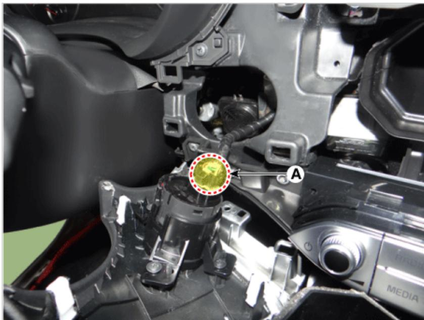
10. Remove the cluster fascia panel (A) by using a remover.
