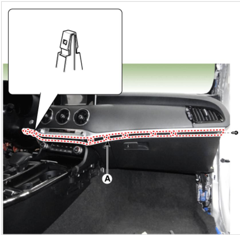
8. Separate the crash pad passenger side panel (A) after loosening the mounting screws.
