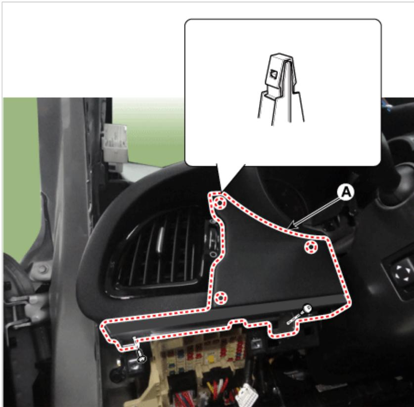
6. Remove the crash pad side cover [RH] (A) by using a remover.
