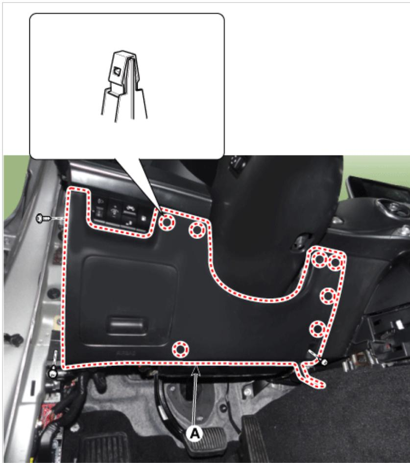
3. Disconnect the crash pad lower switch connector (A).
