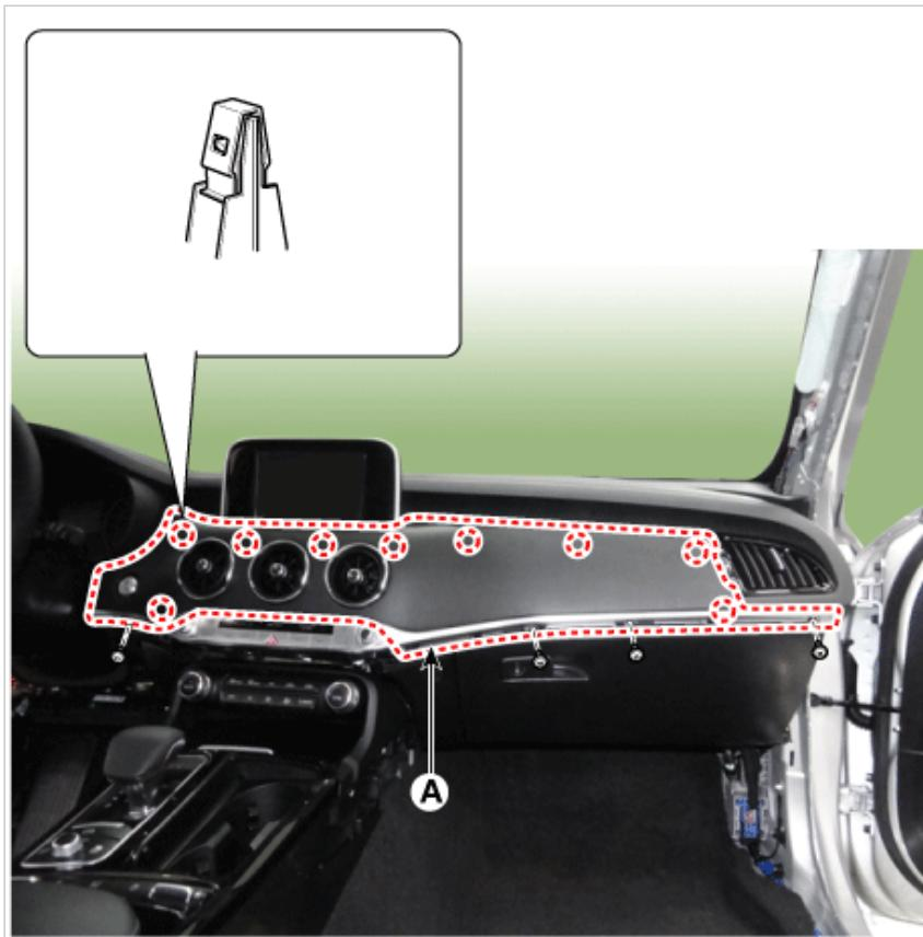
9. Disconnect the start/stop button connector (A) and then remove the crash pad garnish.
