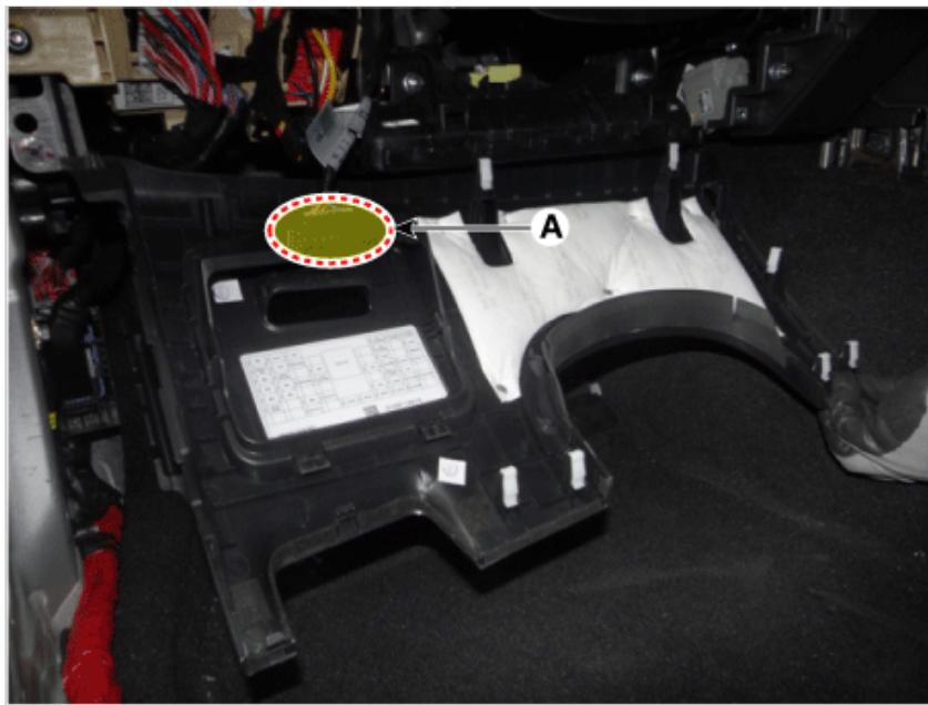
4. Remove the crash pad garnish [LH] (A) after loosening the mounting screws.
