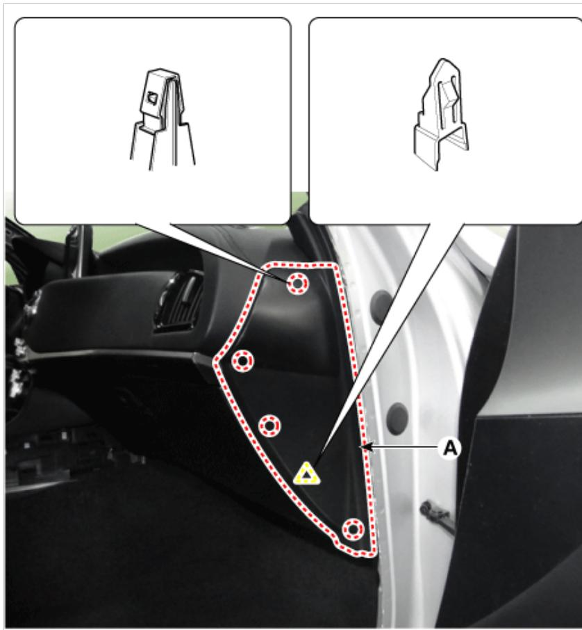
7. Remove the crash pad garnish [RH] (A) after loosening the mounting screws.
