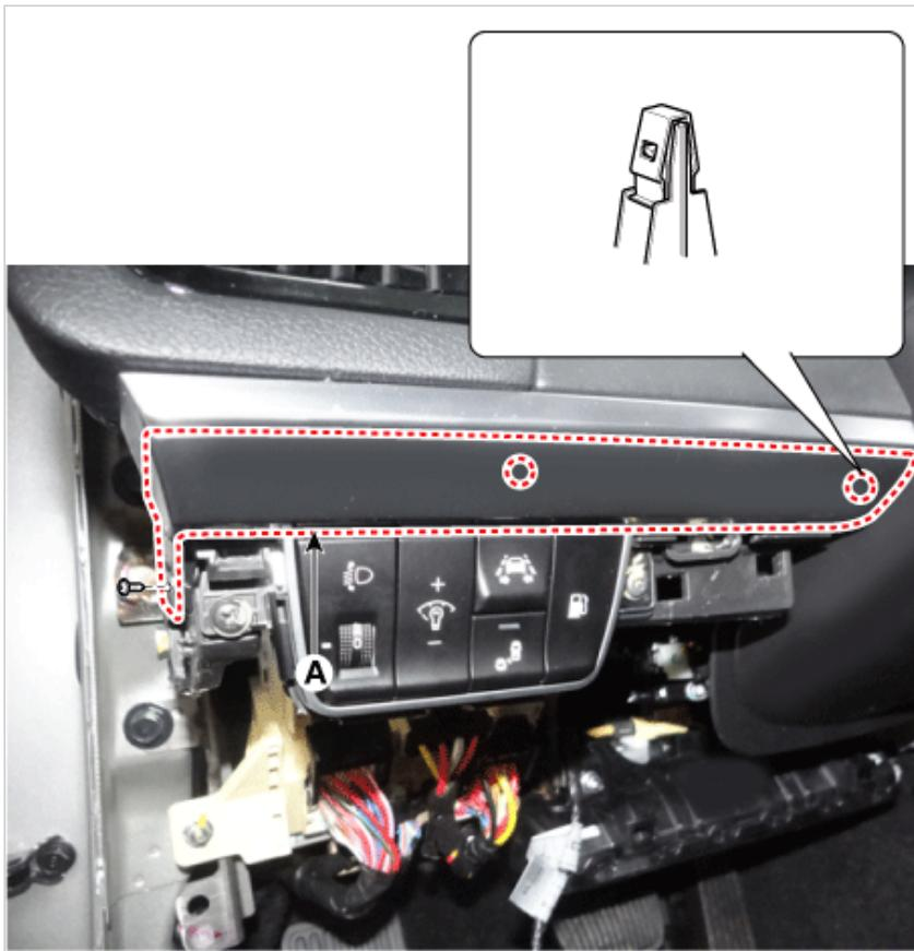
5. Remove the crash pad driver side panel (A) after loosening the mounting screws.
